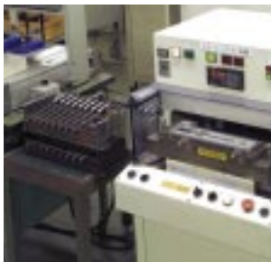
ABS Coolant Proof callipers being tested by air leakage test equipment
