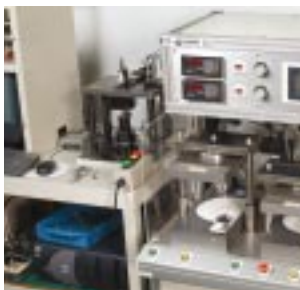
Coolant Proof micrometer being tested by air leakage test equipment
