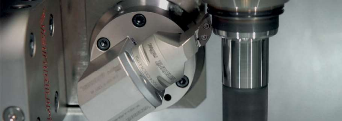
Kugelgelenk (Hartdrehen) Feinschlichten + drall-frei | ball joint (hart part turning) fine-finishing + twist-free
