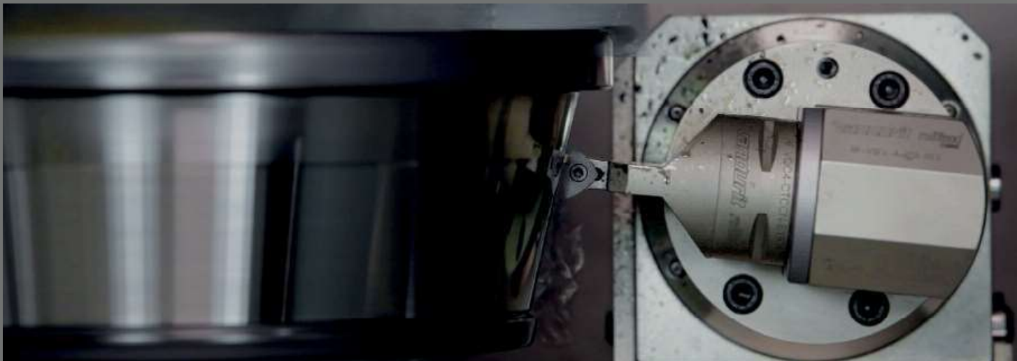
Lagerring (Hartdrehen) Schruppen, Vor- & Feinschlichten | bearing ring (hard part turning) roughing, pre- & fine-finishing
